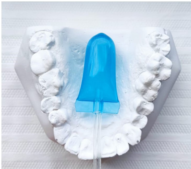
Figure 2. Bulb position during pressure tasks in the posterior tongue region.
